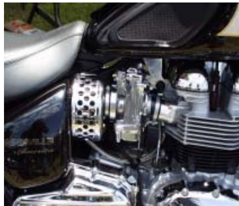
Stage 2 Carb Kit Shown on TBA / Speedmaster
